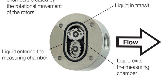
The positive displacement flow technology allows for precise flow measurement of most clean liquids regardless of the media's conductivity. Other liquid properties also have a minimal effect on the performance of this type of meter. Flow profile conditioning is not required, as with alternative flow technology options, making oval gear installations simple to install in tight spaces and at a economical price.
