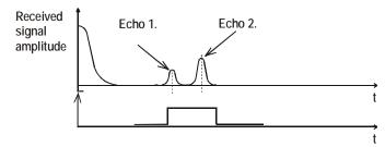
Some applications involve multiple (target + disturbing) echoes even within the measuring window. Basic echo selection will be done by the Quest + software automatically. This parameter influences the echo selection only within the measuring window.
