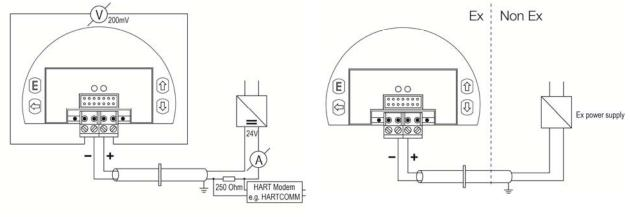
Using HART communication In non-Ex environment Using Ex approved instrument in hazardous environment
