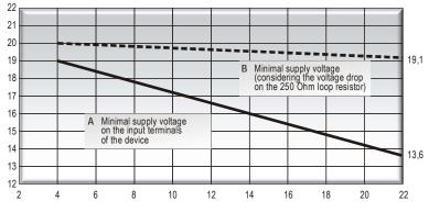
**A**: minimal supply voltage on the input terminals of the device
