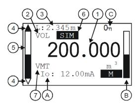
6. Indication of Primary Value simulation. In this case the display and output show the values of the simulation and not the measured values.
