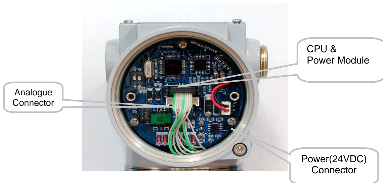
Figure 8.3 Structure of Electronics Module inner Transmitter
