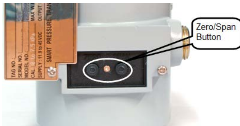
[Figure 5-4 Transmitter Zero/Span configuration Buttons]
