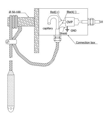
An over-voltage protection (NTB-OVP) should be used with the outdoor-installation. The grounding of the over-voltage protection must be connected to the protective grounding via the shortest path available. Please observe the relevant regulations and safety standards (VDI/VDE).
