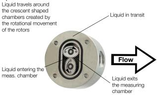
The positive displacement flow technology allows for precise flow measurement of most clean liquids regardless of the media conductivity. Other liquid properties also have a minimal effect on the performance of this type of meter. Flow profile conditioning is not required as with alternative flow technology options making oval gear installations simple to install in tight spaces and at an economical price.
