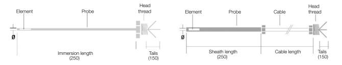
**Note:** Probes are delivered mounted on the housings but may be removed/ interchanged by the customer.
