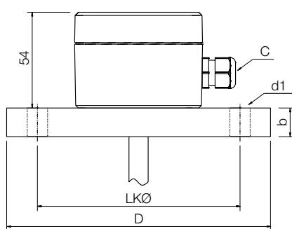
**Flanged process connection acc. DIN EN1092-1 PN16 / ANSI B 16.5 150 lbs with aluminium housing**
