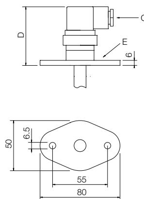
**Oval flange process connection with PA connector DIN 43650 (3 pin), DIN VDE 0627 (6 pin)**
