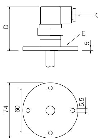
**Round flange process connection with PA connector DIN 43650 (3 pin), DIN VDE 0627 (6 pin)**
